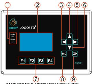
1.LED: From top to bottom: power supply, system start-up, notification, system error
