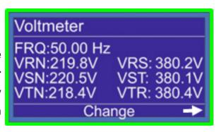
voltage imbalances. In single-phase mode, the controller will only display the input phase R voltage and frequency. By pressing the right key on the Phase Control page, we can separately observe the waveforms of phases T, S, and R. If one of the controller phases is disconnected, this waveform will be displayed as a straight line, making it easy to detect the phase disconnection.
