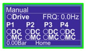
Note that in the Manual Settingspage, the controller will exit the automatic control mode, and after leaving this page, it will return to automatic mode. Additionally, all protections will remain active.
